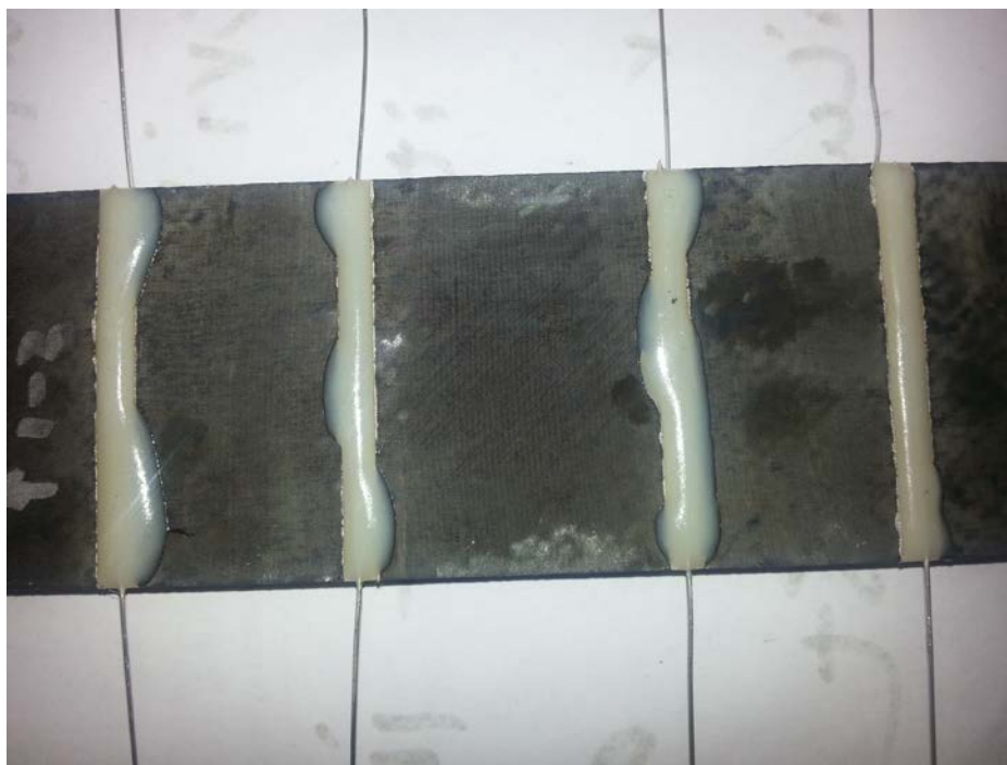
Figure 4.24: Sample 1-8 Bottom Surface after 2 nd Impact
