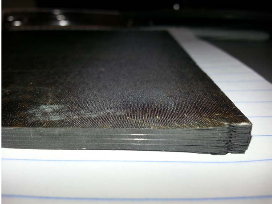
Figure 2.4: Delamination in One of the Samples
