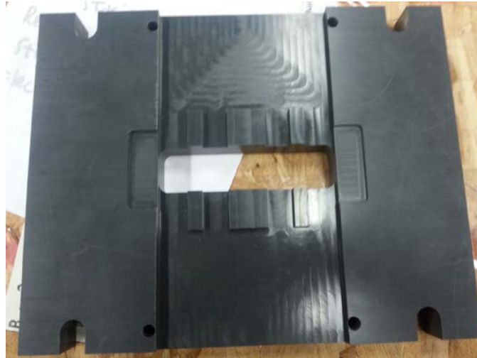
Figure 4.25: New PVC Test Fixture
