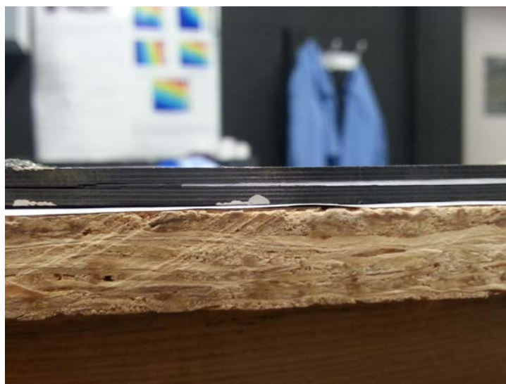
Figure 4.39: Delamination Side 4 of Sample 1-7
