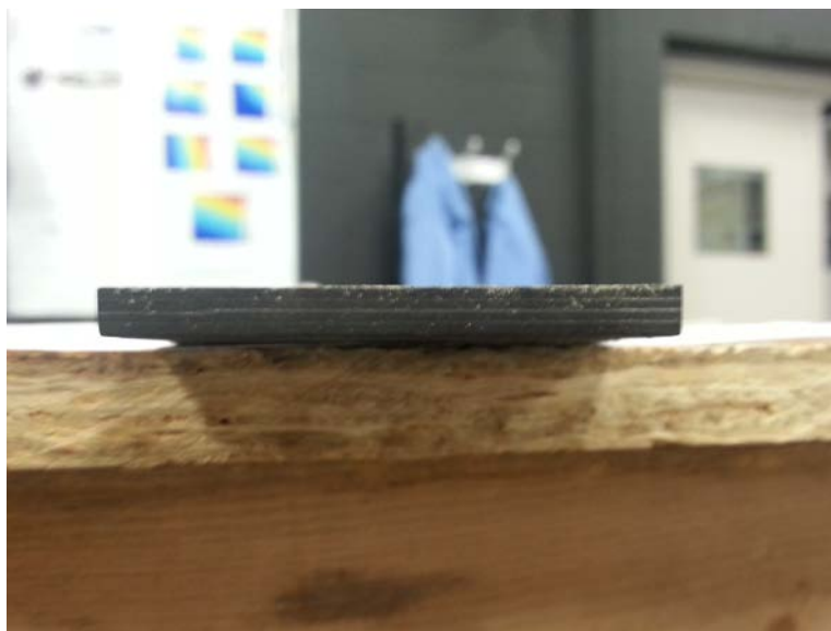
Figure 4.38: Delamination Side 3 of Sample 1-7
