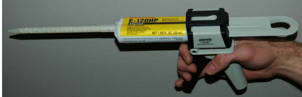
Figure 2.6: Epoxy Applicator (McAndrew, 2009)
