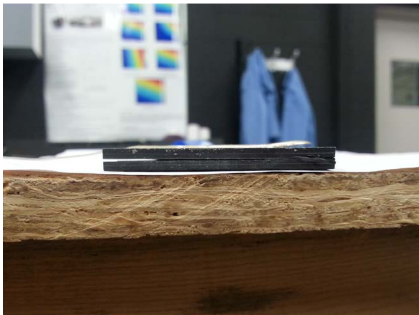
Figure 4.36: Side 1 Delamination of Sample 1-7
